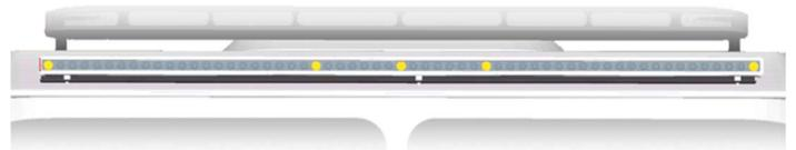
**Body Mounted:** Body mounted scene lights offer ease of setup and simple operation. Often, the operator can switch these fixtures on from the cab. Body mounted scene lights typically come in two variants: "Surface" mounted, or "Recessed"
