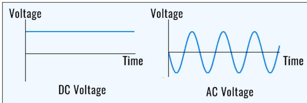
“DC” refers to “Direct Current” and means that the voltage is a constant. Typically, this is 12 volts DC on US fire apparatus. The DC electrical system relies on the Apparatus’ Engine to be running to charge the batteries, which in turn supply power for the items attached to them. DC electrical systems are covered in NFPA 1901 & 1906 Standards, Chapter 13, “Low Voltage Electrical Systems”
