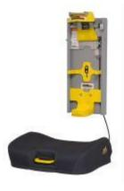
The NFPA states that if SCBA tanks are carried within the crew compartment, they "must be stored in a bracket with a positive mechanical means of holding the SCBA in the event of a 9-G force in any direction." SCBA tanks can become a deadly, pressurized, flying projectile capable of injuring occupants. Keeping them secured is a key safety consideration.
