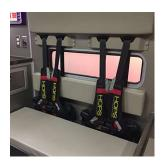
**4-POINT SEAT BELT HARNESS –** This 4-point retractor restraint system includes a central buckle, which provides occupants greater mobility. It is used primarily in the ambulance and EMS applications.
