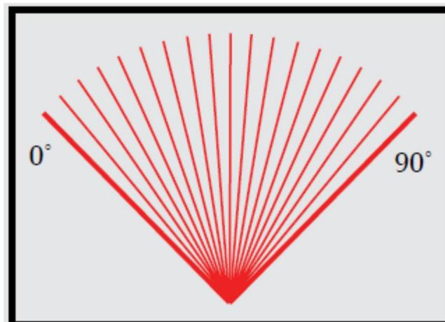
Each Zone on a Large or Small Apparatus consists of 19 data points (10,000 candela-sec./min.) where light energy is measured. See illustration above.
