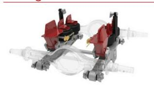
The Air Over Walking Beam Air Ride suspension has a Non-Torque Reactive Air Suspension on top of the walking beam to optimize the relationship of ride quality, roll stability, and off-road mobility and traction. These systems use an air spring to isolate road inputs and height control valves to maintain a constant ride height. Air springs have internal rubber up stops
