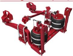
Torque Reactive Air ride suspensions are available in both single and tandem axle configurations. These systems use an air spring to isolate road inputs and height control valves to maintain a constant ride height. Torque reactive air ride suspensions are considered entry level air rides. Torque reactive air suspensions connect solid to the axle and do not use a longitudinal upper torque rod. This causes the axle to swing through an arc. The suspension geometry
