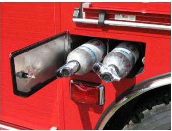
Additional cylinders can be mounted in the truck compartments (with proper depth behind the door).
