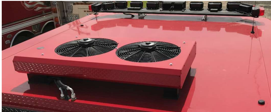
Roof Mounted Condensor
