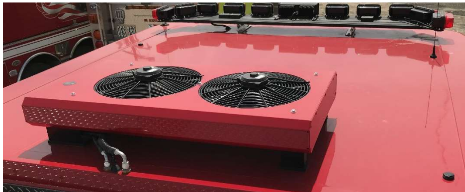
Roof Mounted Condensor
