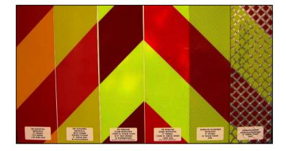
When specifying retroreflective striping on fire apparatus whether the installation is performed by the apparatus manufacturer, a third party installer or installing it yourself, NFPA compliance should be specified. This should cover the technical aspect of retroreflectivity.
