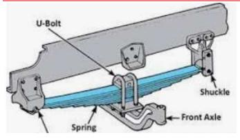
This system historically was the most common in fire apparatus so has the highest population in the field. A multileaf features multiple leaves and has a step-down effect with each leaf being progressively shorter than the one above it.
