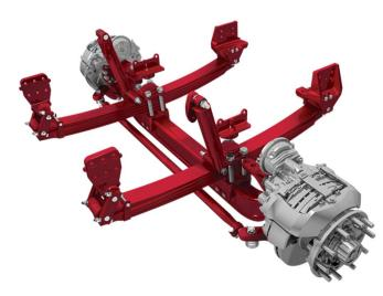
A parabolic taper-leaf spring suspension has fewer leaves and tapers at each end. The parabolic springs will have spacers to separate them so will typically only contact at the ends to reduce contact and friction between the leaves. This type of system is becoming the standard beam based front suspension in fire apparatus.
